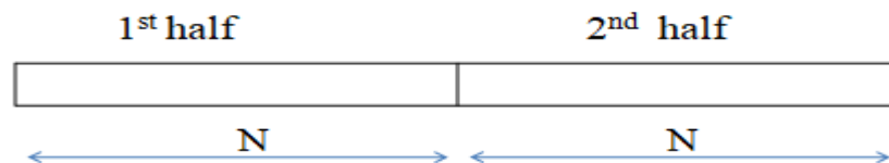
Fig. 1.7. An input buffer in two halves.
