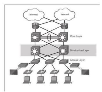
The core layer is also referred to as the network backbone. The core layer consists of high-speed network devices such as the Cisco Catalyst 6500 or 6800. These are designed to switch packets as fast as possible and interconnect multiple campus
