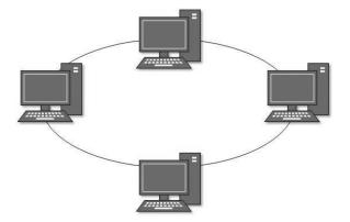
Failure of any host results in failure of the whole ring. Thus, every connection in the ring is a point of failure. There are methods which employ one more backup ring.
