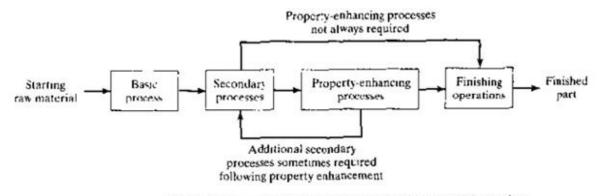
Typical sequence of processes required in part fabrication.
