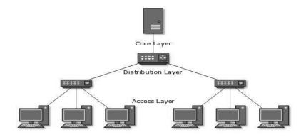
All neighboring hosts have point-to-point connection between them. Similar to the Bus topology, if the root goes down, then the entire network suffers even though it is not the single point of failure. Every connection serves as point of failure, failing of which divides the network into unreachable segment.
