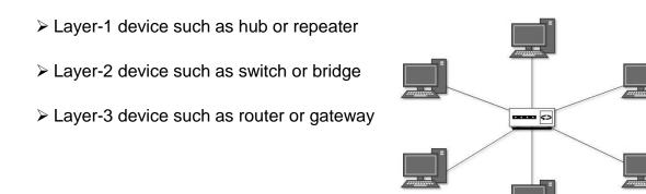
As in Bus topology, hub acts as single point of failure. If hub fails, connectivity of all hosts to all other hosts fails. Every communication between hosts takes place through only the hub. Star topology is not expensive as to connect one more host, only one cable is required and configuration is simple.
