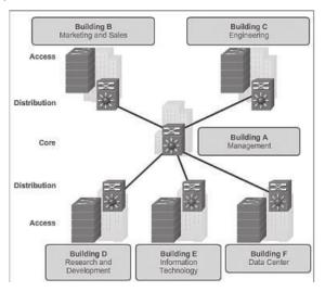
In a LAN environment, the access layer highlighted grants end devices access to the network. In the WAN environment, it may provide steelworkers or remote sites access to the corporate network across WAN connections. The access layer serves a number of functions, including:
