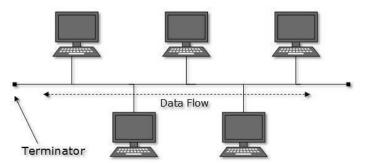
Both ends of the shared channel have line terminator. The data is sent in only one direction and as soon as it reaches the extreme end, the terminator removes the data from the line.
