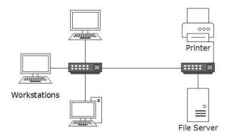
LANs are composed of inexpensive networking and routing equipment. It may contains local servers serving file storage and other locally shared applications. It mostly operates on private IP addresses and does not involve heavy routing. LAN works under its own local domain and controlled centrally.
