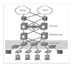
The distribution layer aggregates the data received from the access layer switches before it is transmitted to the core layer for routing to its final destination.
