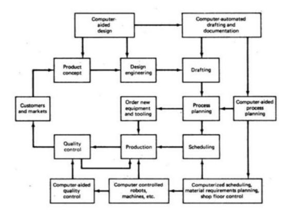
Fig: Implement of CAD/CAM in Product life cycle
