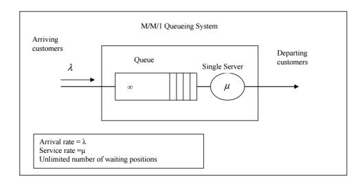
Rate transition diagram for an M/M/1 Queueing System
