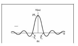
$$X(j\omega) = \int_{-\infty}^{\infty} x(t)e^{-j\omega t}dt = \int_{-T_1}^{T_1} 1e^{-j\omega t}dt = 2\frac{\sin\omega T_1}{\omega}$$
