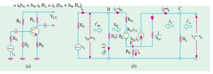
$$\therefore \qquad r_{in} \quad \frac{v_{in}}{i_b} \quad h_{ic} \quad h_{fe} R_L$$
