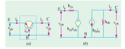
Its ac equivalent circuit employing h-parameters is shown in Fig. (b).
