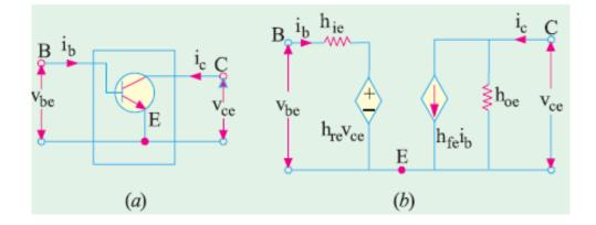
Input signal source across its input terminals and load resistance across output terminals may be connected
