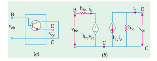
• Input signal source across its input terminals BC and load resistance across output terminals EC may be connected in order to get a CC amplifier
