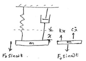
The type of vibration which occurs under the influence of external force, is called "FORCED VIBRATION". The external force is called External excitation.
