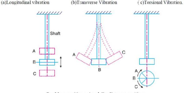
B = Mean position ; A and C = Extreme positions.(a) Longitudinal vibrations.(b) Transverse vibrations.(c) Torsional vibrations.
