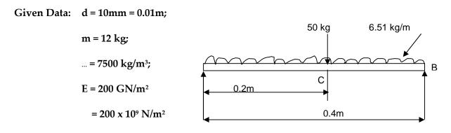
To find Whirling speed by (i) neglecting the mass of the shaft, and (ii) considering the mass of the shaft
