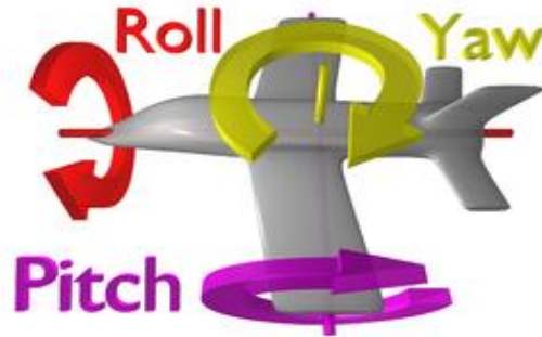
Fig 9 .Attitude degrees of freedom for an airplane.
