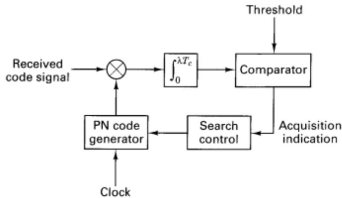
**Figure 4.4** Direct-sequence serial search acquisition.
