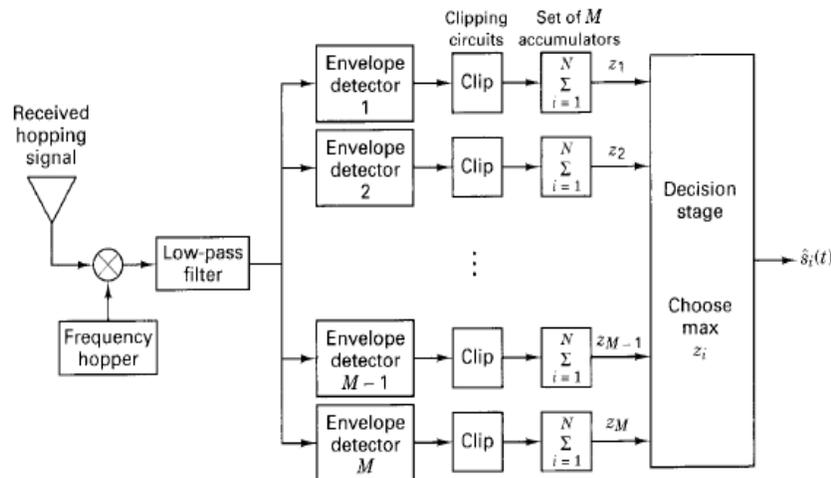
Figure 4.1 FFH/MFSK demodulator.
