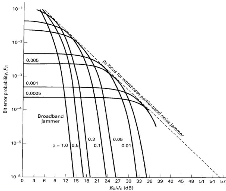
**Figure 4.12 Partial band noise jammer (FH/BPSK signaling)**
