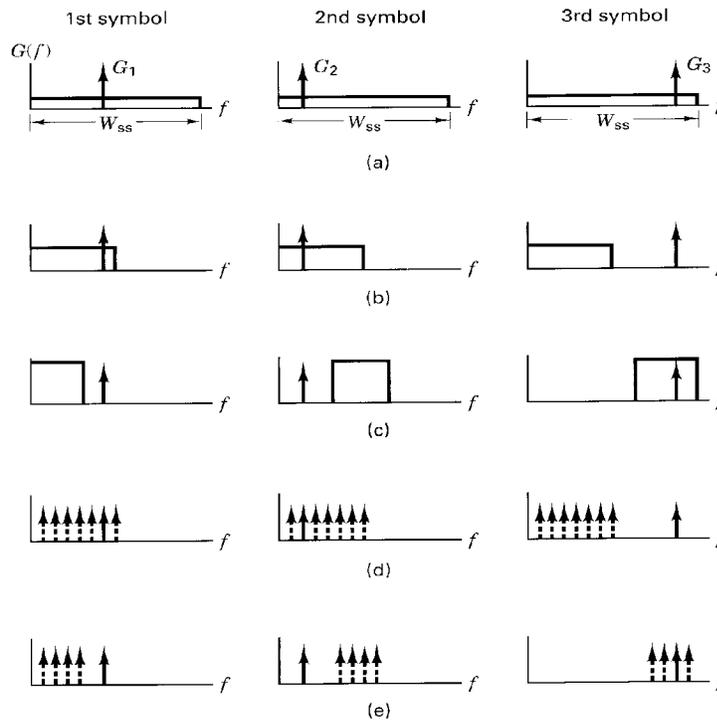
Figure 4.10 Jammer waveforms. (a) Full-band noise. (b) Partial-band noise. (c) Stepped noise. (d) Partial-band tones. (e) Stepped tones.
