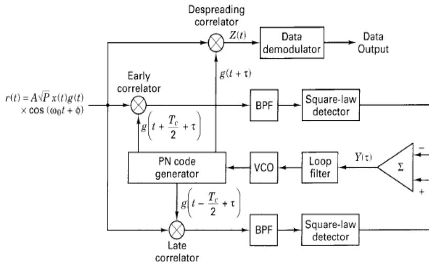
Figure 4.7 Delay-locked loop for tracking direct-sequence signals.
