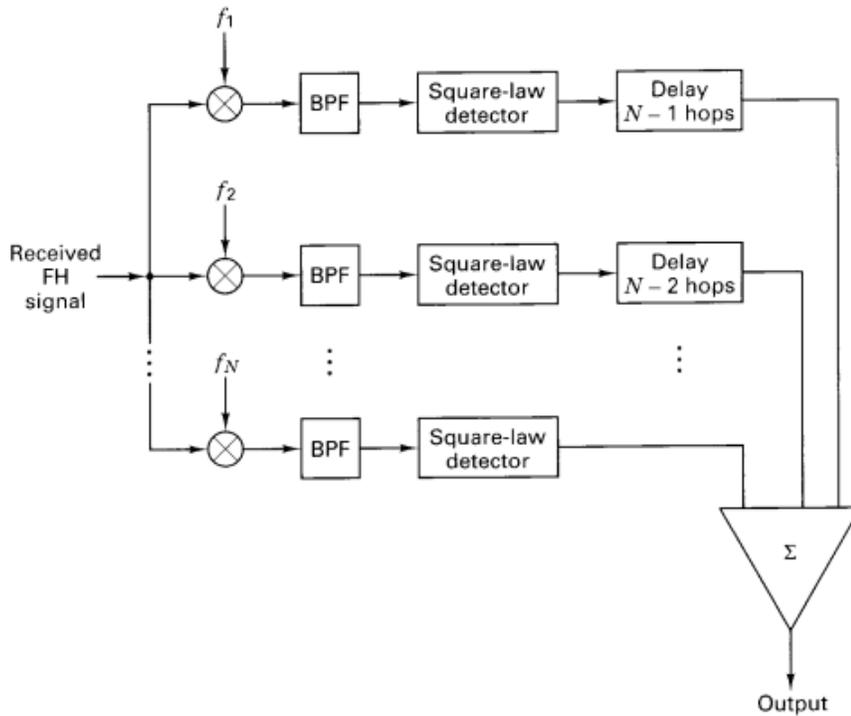
**Figure 4.3** Frequency hopping acquisition scheme.
