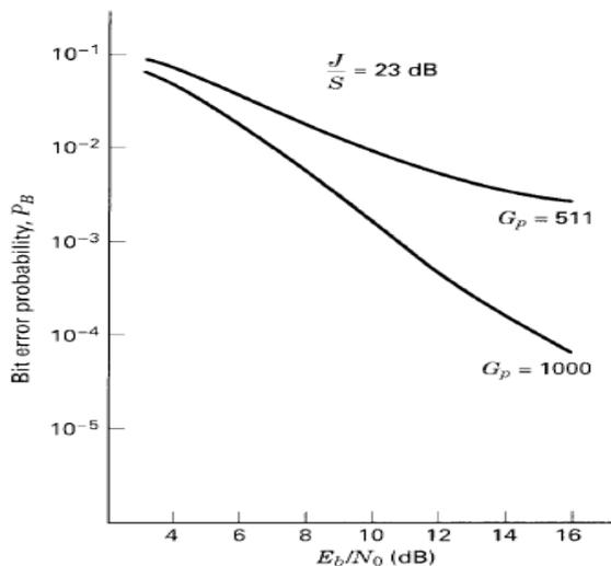
**Figure 4.11 Bit-error probability Versus  $E_b/N_0$  for a given  $J/S$  ratio**
