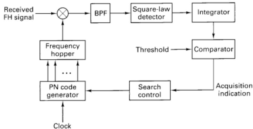
**Figure 4.5** Frequency hopping serial search acquisition.
