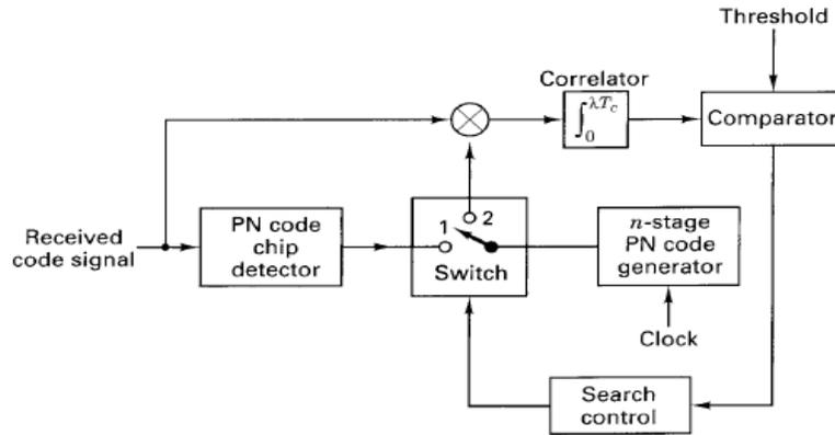
Figure 4 Rapid acquisition by sequential estimation.
