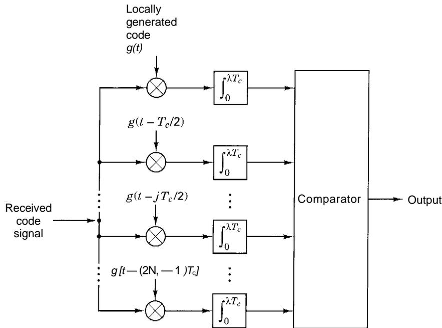
**Figure 4.2** Direct-sequence parallel search acquisition.
