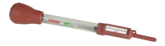
The specific gravity of an electrolyte can be found out using Hydrometer. It consists of a rubber bulb at the top. A graduated float is placed inside this glass tube. The rubber bulb is attached to the top and a nozzle is attached to this bottom of the glass tube.
