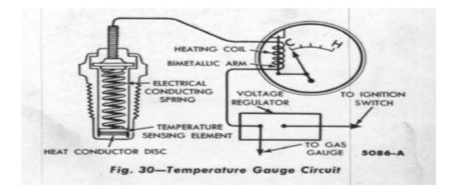
This is used to check the temperature at the coolant used in the engine. Based on the construction an functioning the entire part of the guage can be separated into two section. They are temperature plug and temperature gauge
