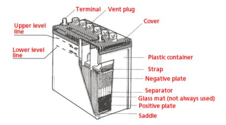
There are two types of plates in Battery, They are i) Positive plates ii) Negative plates. These plates are placed across each other and are supported by a Rectangular gird. The Positive plates are made of Lead Pr Oxide(Pbo<sub>2</sub>), the negative plates are made of Spongy lead and the grid is made of lead Antimony Alloy. Generally the no of negative plates are more than the number of positive plates. For eg: for a cell made of 19 plates there will be 10 negative plates and 9 positive plates.
