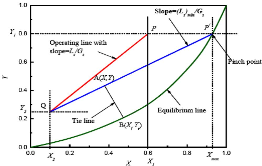
Graphical determination of  $(L_s)_{min}$  for absorption.
