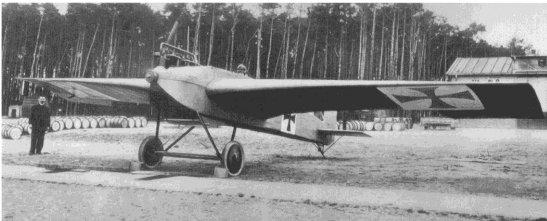
The pioneering Junkers J 1 all-metal monoplane of 1915, the first aircraft to fly with cantilever wings
