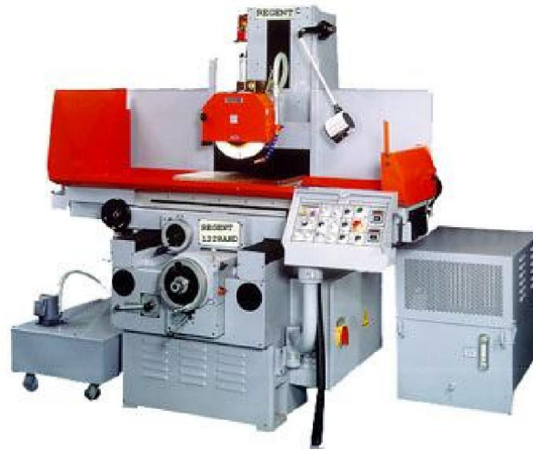
Surface grinder with horizontal spindle and reciprocating worktable.
