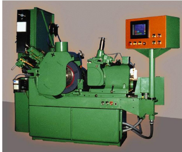
External centerless grinder.
