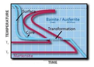
The red lines form the transformation diagram and blue line denote the process. In this case the component which had an austenitic structure was cooled to just above Ts temperature; held at that temperature until the transformation was complete and then cooled further to the room temperature.
