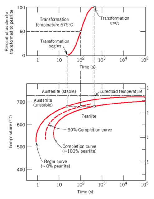
Then these transformation start times and transformation end times are plotted for different temperatures as shown. These points, when joined, give us the TTT diagrams. For continuous cooling, the time required for the transformation to begin and end is delayed. Thus the TTT diagram's curves are shifted to longer times and lower temperatures.
