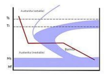
In the above given Time-temperature transformation (TTT) diagram. The red line shows the cooling curve for austempering.
