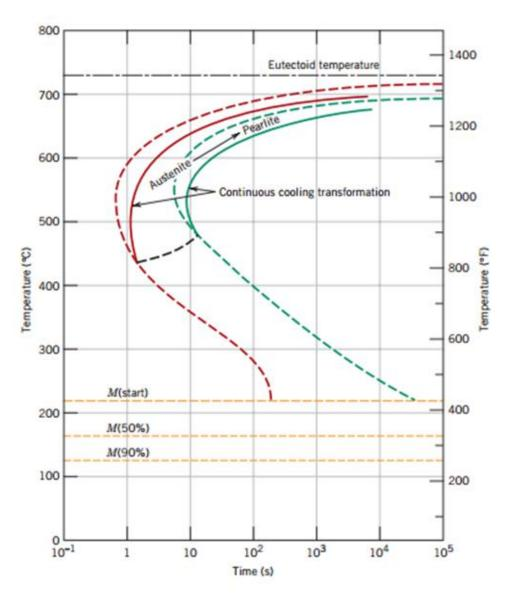
The dashed lines form TTT diagrams and the solid lines form the CCT diagrams. It can be seen that CCT diagram can be obtained by moving the TTT curves a little to the downward right.
