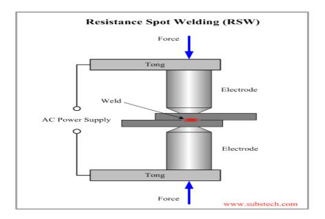
**Spot Welding** is a Resistance Welding (RW) process, in which two or more overlapped metal sheets are joined by spot welds.
