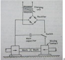
the butt welding of bars, rods, tubes and pipes.
