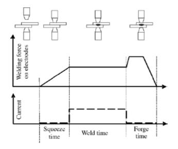
HOW THE ELECTRODE FORCE IS OBTAINED
