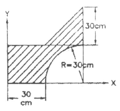
Divide the diagram in to three sections with their individual centroid
