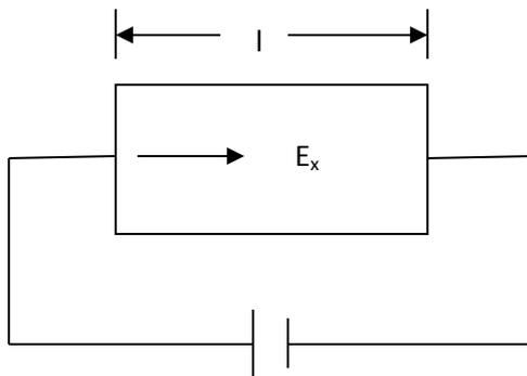
The ability of an electron to drift under the influence of electric field is called Mobility.
