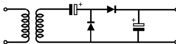
**Diode voltage doubler circuit**
