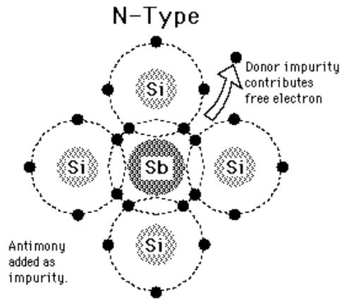
Formed when a pentavalent impurity is added to intrinsic material.
