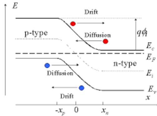
When the N and P-regions are brought into contact, the electrons would flow from regions of higher Fermi-energy to regions of lower Fermi energy and holes would flow in the opposite direction.
