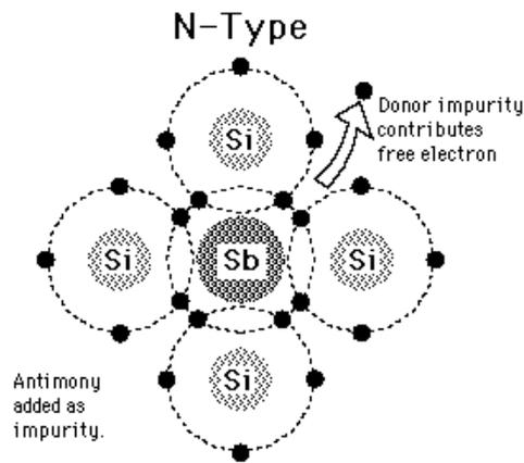
Formed when a pentavalent impurity is added to intrinsic material.
