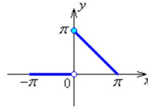
$$a_0 = \frac{1}{\pi} \int_{-\pi}^{\pi} f(x) dx = \frac{1}{\pi} \int_{-\pi}^0 0 dx + \frac{1}{\pi} \int_0^{\pi} (\pi - x) dx$$
