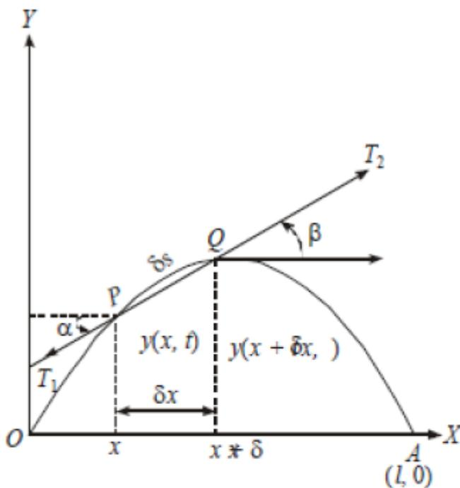
$$\Rightarrow \quad \frac{\partial^2 y}{\partial t^2} = \frac{T}{m} \frac{\partial^2 y}{\partial x^2}$$
