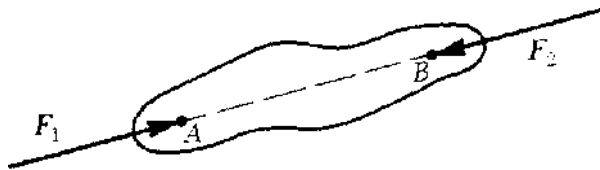
Figure 1.2(A) A two-force member. The resultant force and the resultant moment both equal Zero.
