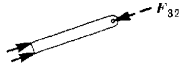
Figure 1.1(E) Free body diagram of part of a link.
