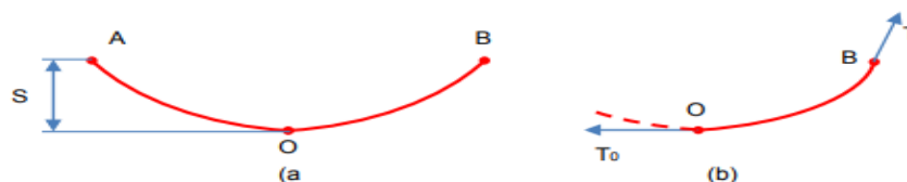
Figure 23. Conductor suspension between two supports
