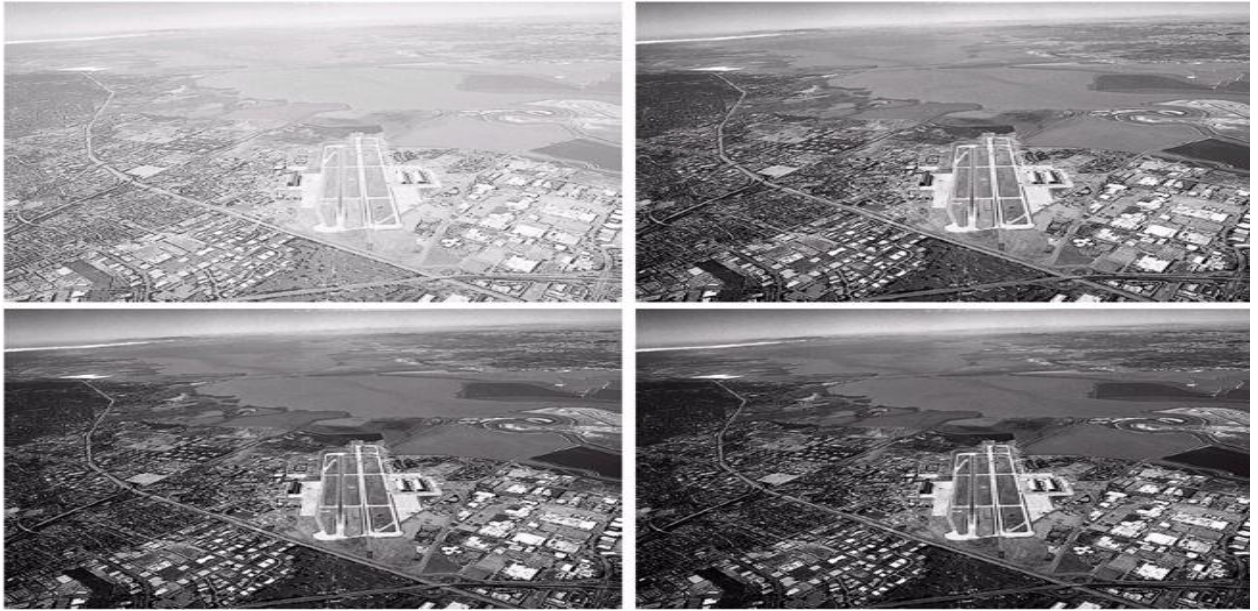
(a) Aerial image (b)-(d) results of applying the transformation with c=1 and Y=3, 4 and 5 respectively
