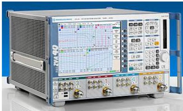
Network analyzers are used mostly at high **frequencies**; operating frequencies can range from 5 Hz to 1.05 THz. Special types of network analyzers can also cover lower frequency ranges down to 1 Hz. These network analyzers can be used for example for the stability analysis of open loops or for the measurement of audio and **ultrasonic** components.
