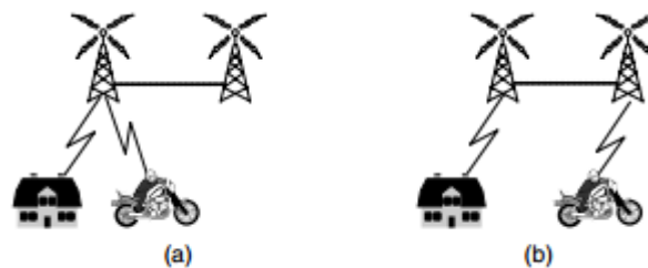
Figure 1.29 Mobile phone handover (a) Before (b) After
