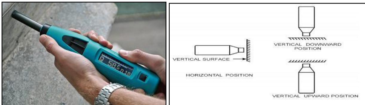
Rebound Hammer Positions for Testing Concrete Structure
