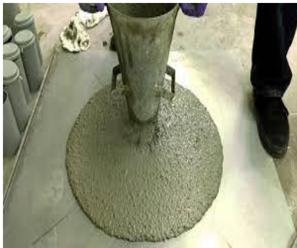
Flow table test apparatus
