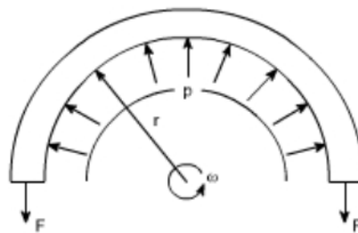
Fig 19.1: Thin ring rotating with constant angular velocity \omega
