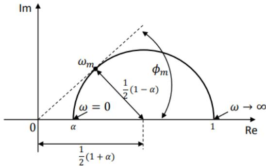
Polar plot of a lead compensator:
