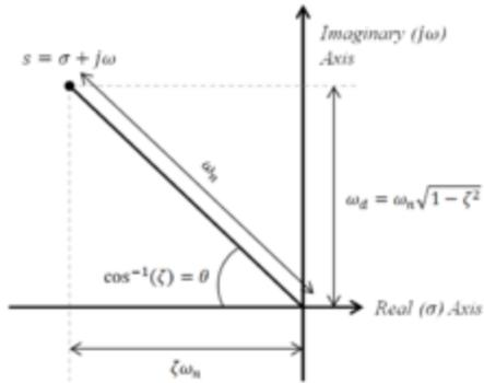
Effect of pole location on a second order system's natural frequency and damping ratio.
