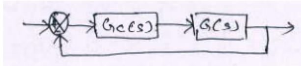
A Controller with transfer function  $G_c(s)$  can be introduced in cascade with open loop transfer function,  $G(s)$  to modify the transient and steady state response of the system.
