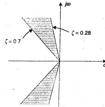
For the antenna position control system, gain is the only adjustable parameter. If we increase gain, settling time will decrease. At the same time, peak overshoot will increase, this indicates the increase in peak overshoot. Thus by merely increasing gain, we cannot improve both transient and steady-state error specifications. We need to add additional components to the system. These are called compensators. It will allow improvement of both transient and steady-state specifications.
