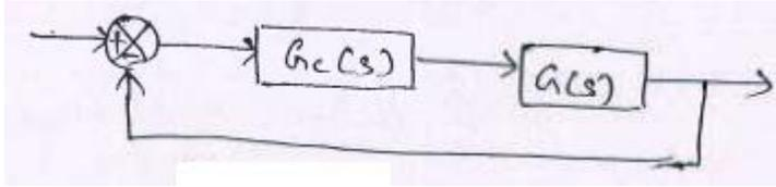
Open loop transfer function of compensated system,  $G_o(s) = G_c(s) \times G(s)$
