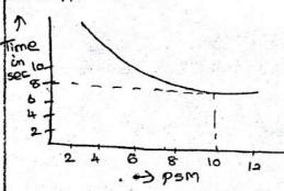
For a relay, a curve showing relation between time and plug setting multiplier is provided which is abled time / ps. My curve. Using this curve and time-setting multiplier, the actual time of operation of a relay can be obtained.
