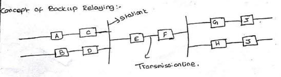
relays GD, G&H are primary relays relays A.B. I. I are backup relays
