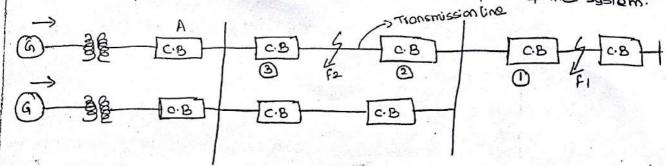
If fault F2 arous on Honsmission line then the C.B's @ 4 (3) should apperate and disconnect the line from the romaining system. It should not operate for fault p, which occurs beyond its protection zone.
