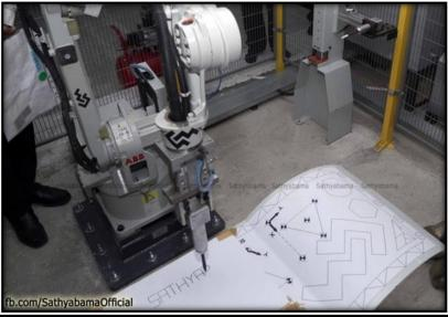
The Center of Excellence for Robotics and Automation was established in 2019 to cater the automation knowledge needs in the field of robotics and Artificial intelligence. This center has an exclusive Industrial robot of ABB IRB 1520 (6 axis) to perform operations, programming, and advanced control systems.
