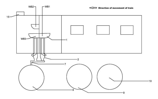
Scheme of Wash basin Water treatment in Railway Compartment
