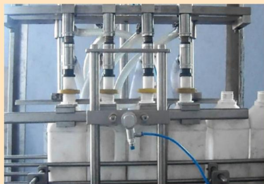
Bottle filling machine funded by Sathyabama
