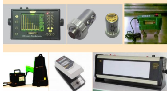
Digital Ultrasonic Flow Detector, Magnetic Particle Testing Equipment, calibration blocks and flawed specimens, Dye penetrant Testing kit & flawed specimens, Radiography accessories funded by Sathyabama
