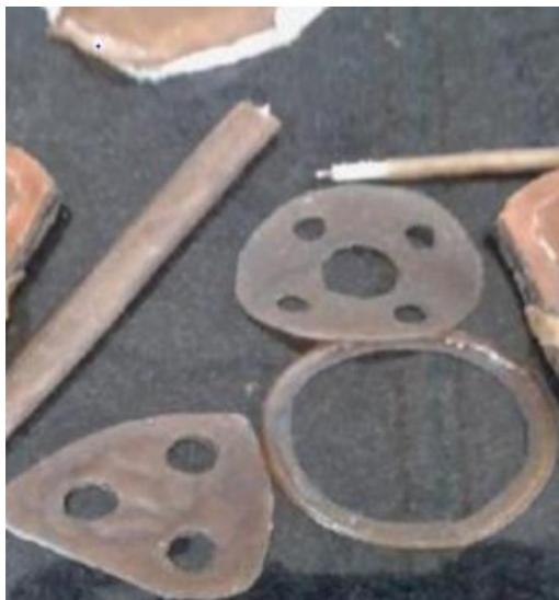
**Automobile components made from algal reject**
